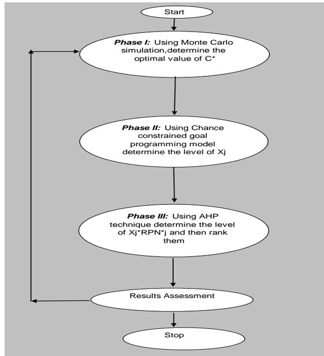
Fig 3. The three-phase method of system risk analysis
