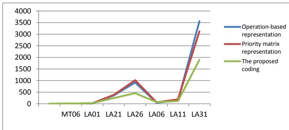
Fig 11. The Average Computational Time for Different Job Shop Problems
