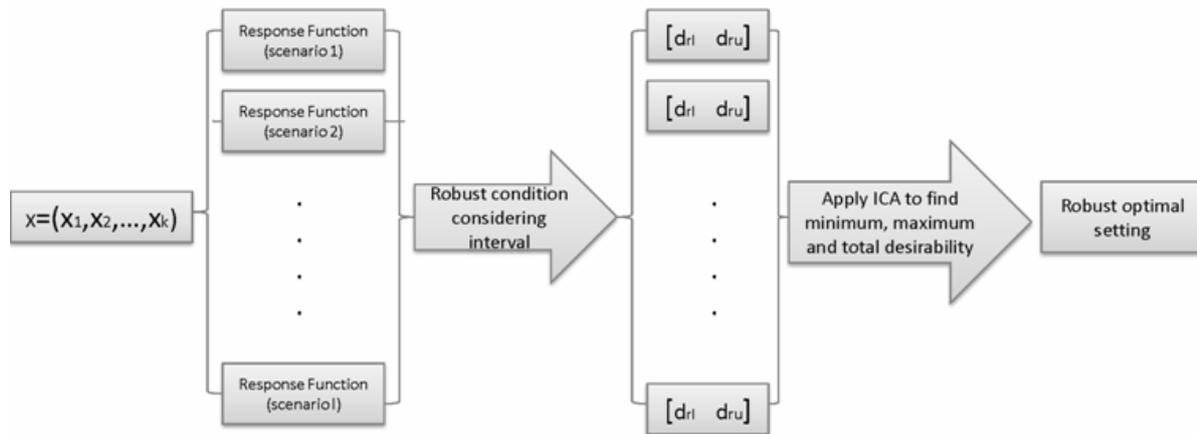
Fig. 2. Flow chart of the proposed robust optimal desirability approach
